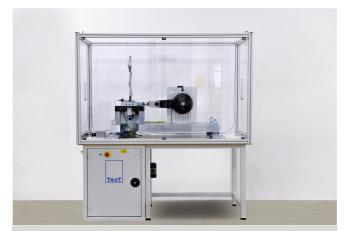
Vibration testing machines acc. to "Junker" DIN 65151
