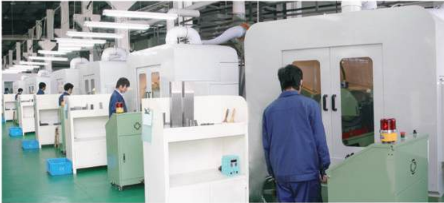
● IMPORTED CNC MACHINERY SPECIAL GRINDING EQUIPMENT FOR MACHINE SCREW PLATE AFTER HEAT-TREATMENT
